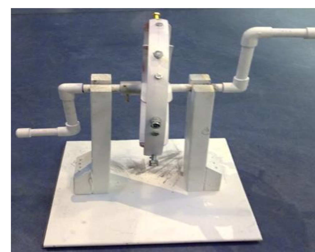
Figure 4: The Flywheel Brass bolts were added to increase the weight and inertia.
