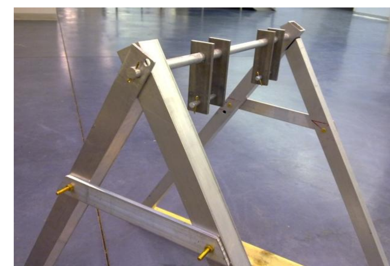
Figure 5: The Triangular Supporting Structure Aluminum beams and brass bolts were used to construct the sides.
