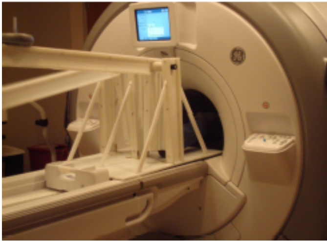
Figure 13: Testing of the prototype within the WIMR MRI bore
