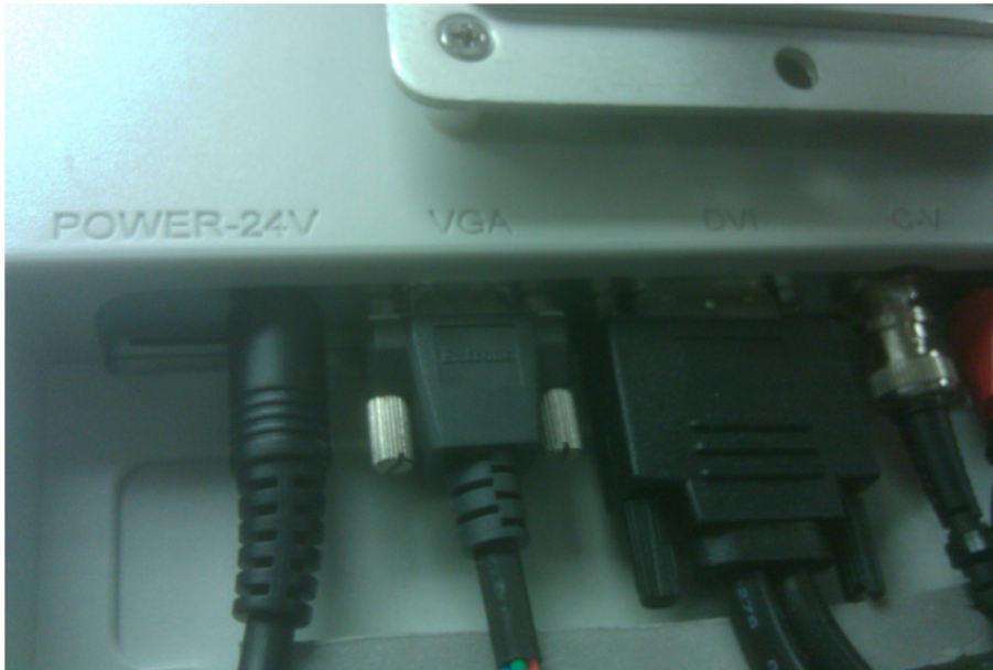
Figure 4: Operating room screen video inputs
