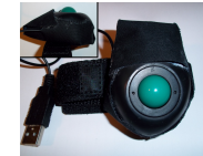
Figure 7: Trackball prototype that attaches to laparoscope
