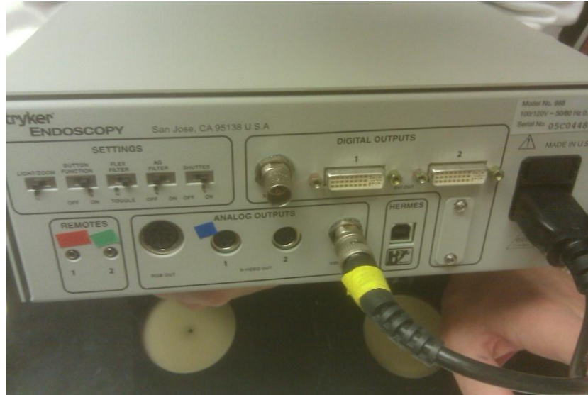
Figure 3: Camera control box outputs. Digital outputs are limited to DVI, while analog outputs may be S Video or BNC
