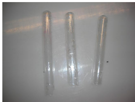
Fig. 9 The fracture pattern of the glass ampoules broken using our final prototype
