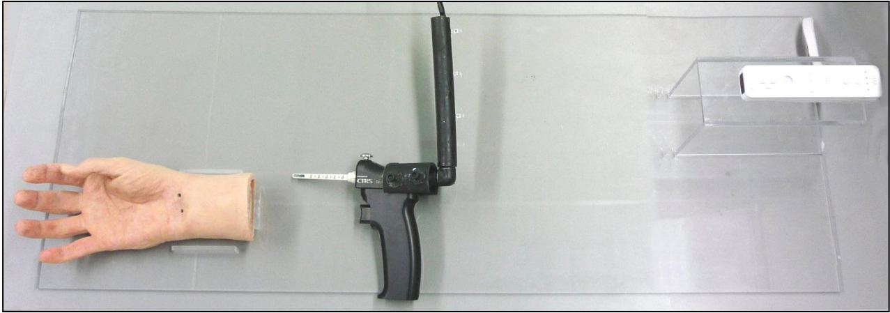
Figure 5. Final prototype with the acrylic platform housing (from left to right) the hand model, the endoscope with blade attachment, the LED circuit, and the receiver.
