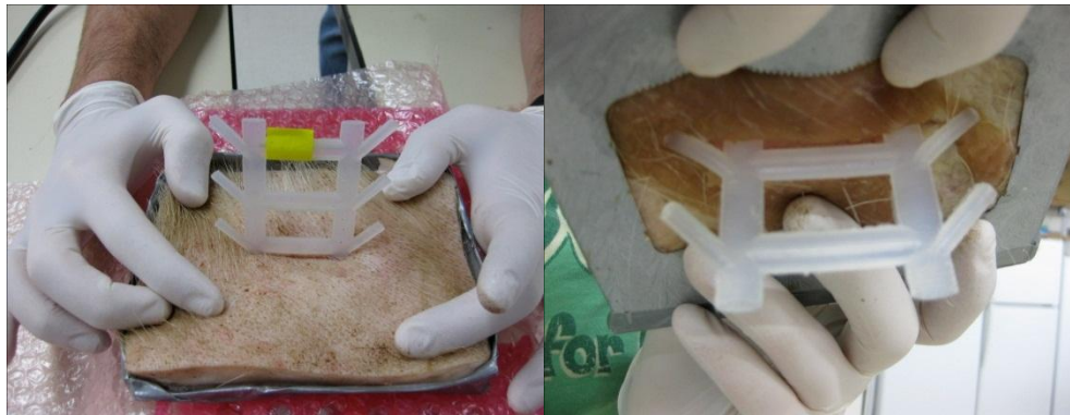
Figure 4: Pig abdominal tissue testing showing LAIP inserted into a 2" surgical incision. Note manner in which the angled posts anchor once inserted through the pig tissue. Both insertion and removal forces were quantified using this mock abscess model.
