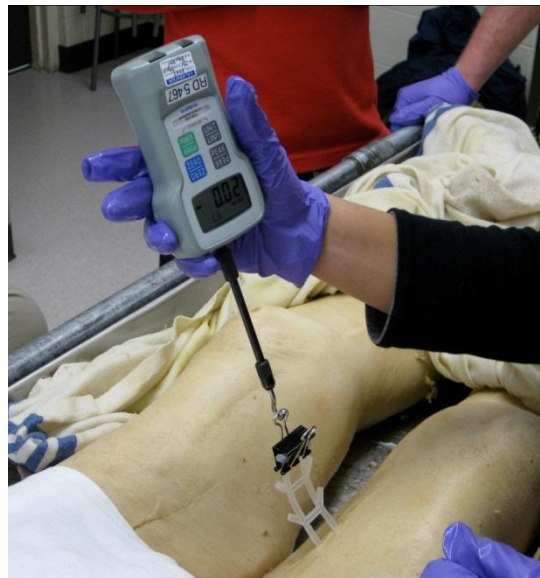
Figure 3: Cadaver thigh model testing for quantification of removal ladder drain variant removal force. A Shimpo FGE-50X digital tensile force gauge was used to record peak force for all ladder drain variants ( n = 3 ).
