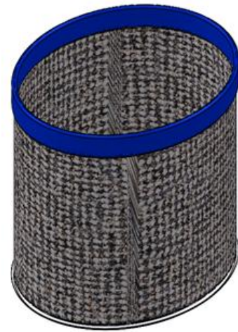
Figure 6: Design 2 is a revised Alexis® device that has the features of Design 1 as well as a supportive mesh structure surrounded on both sides by the polyurethane tube.
