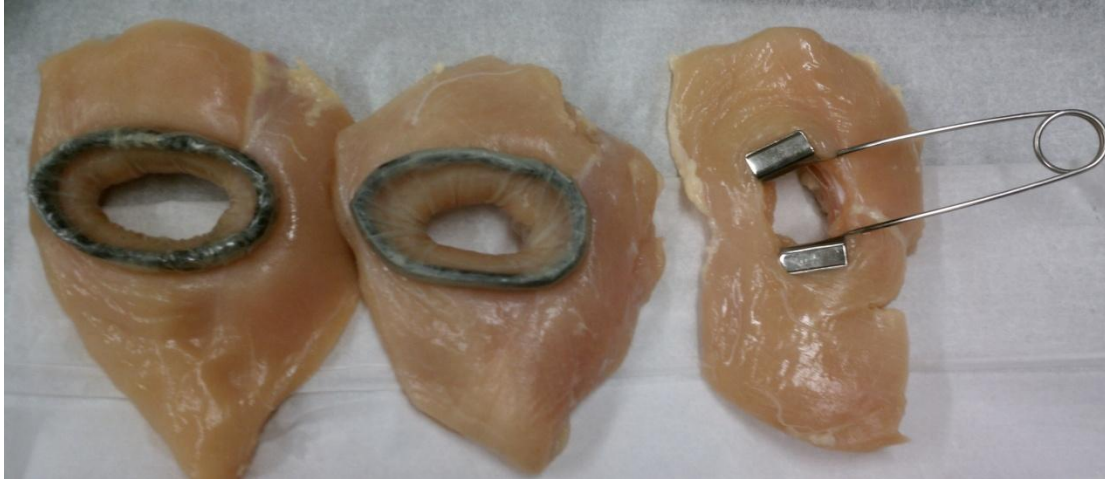
Figure 10: The function of the metal spring retractors and the revised Alexis prototypes were tested in chicken breast. From left to right, revised Alexis 1 (polyurethane tubing and ring), revised Alexis 2 (synthetic nitrile tubing, polyurethane ring), large metal retractor.
