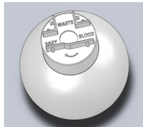
Figure 7: A SolidWorks® top view of the final base to be fabricated in polypropylene.
