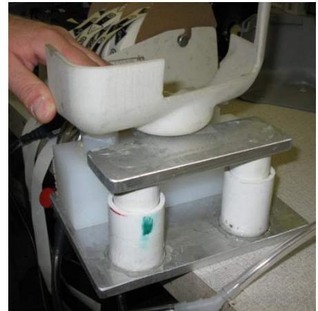
Figure 2: Template and Spring System The template is fastened to the spring support system. The spring allow for the template to move up and down.
