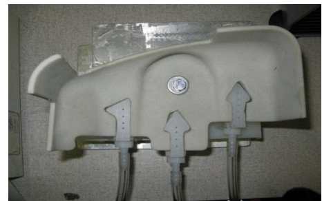
Figure 3: Template with Pedestals The pedestals sit directly below the template, and protrude into the arrow cutouts.
