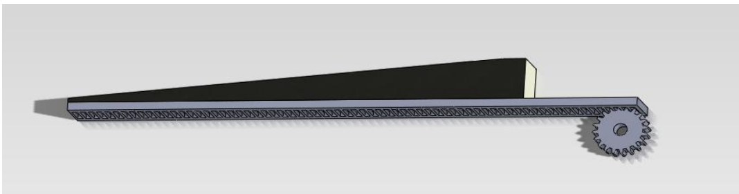
Figure 11: Solidworks representation of rack and pinion system attached to attenuating wedge.
