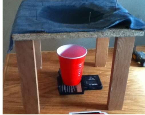
Figure 12: The general testing setup consists of the material held firmly in place and a cup to catch the leaked water.
