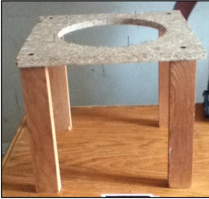
Figure 11: The testing structure used. It stands 30 cm high and the hole is 12 cm in diameter.
