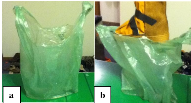
Figure 16: To test the water resistance properties of the boot, a green bag (a) was filled with approximately 400 mL of water and the boot was placed inside (b) and shaken.
