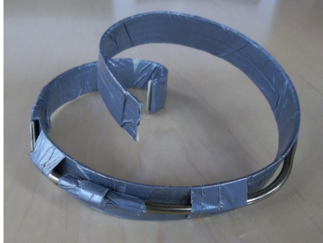
Figure 14. The reinforcement bar placed on the backside of the coil design.
