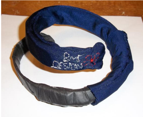
Figure 7. Reinforcement bar placed on the backside of the coil design.
