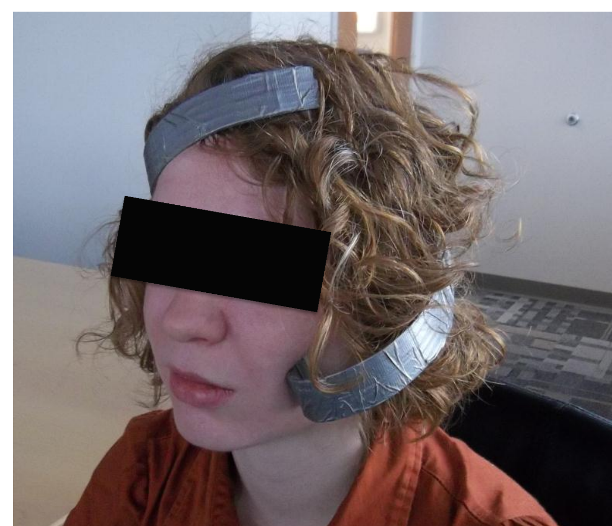
Figure 10: Coil prototype; capable of applying 6.7 N force.
