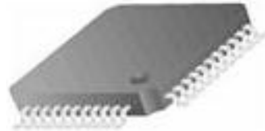
Figure 9: The Atmel controller is specified in a TQFP- 44 packaging.
