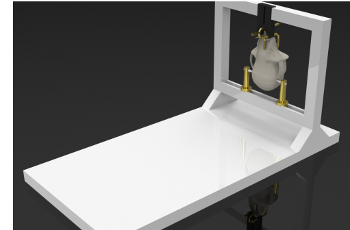
Figure 4: Redesigned head holder with stabilized Rhesus Monkey skull. Photo courtesy of Gabriel Bautista.
