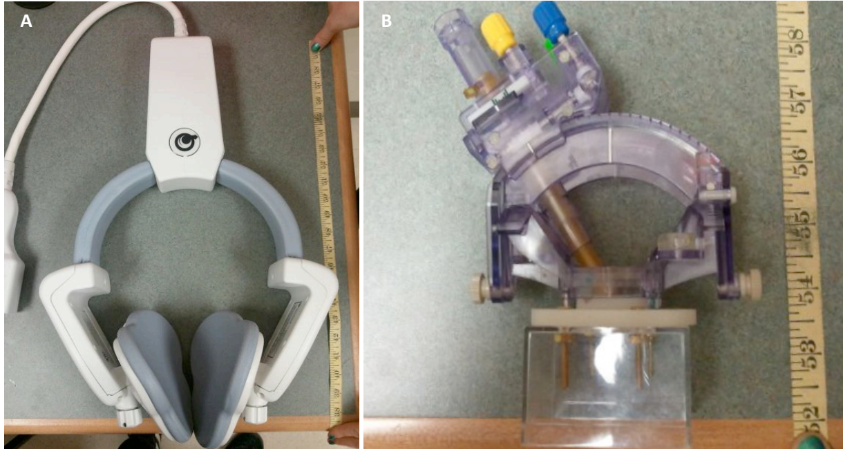
Figure 3: A. Photo of carotid coils. B. Photo of MRI Interventions port. Photos courtesy of Kevin Beene.
