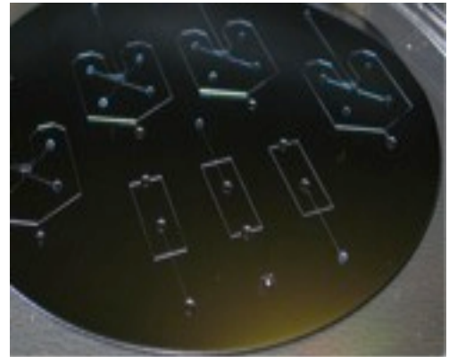
Figure 2: Silicon wafer with SU-8 channel features (Image retrieved from: www.blogs.rsc.org/chipsandtips/2008/04/22/integrated-reservoirs-for-pdms-microfluidic-chips/ )
