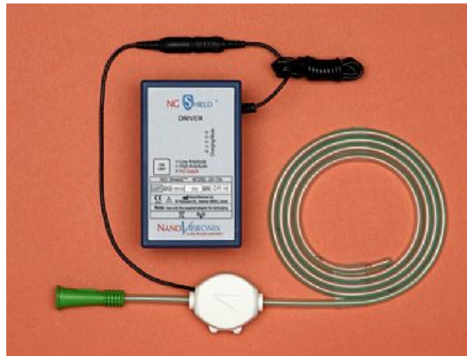
Figure 2: A NG-Shield device that generates acoustic surface vibrations to decrease the friction of the nasogastric tube upon insertion.
