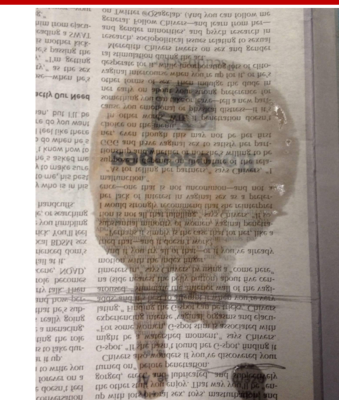
Figure 9 – The silicone oil was sprayed onto a news paper held against the wall. The area of the spray was measured. The shape of spray area was idealized to be an ellipse.
