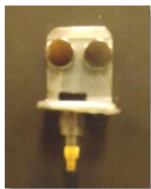
Figure 4. Method of attachment. 4 neodymium magnets were used to secure the accelerometer to an I-beam below the belt of the treadmill. An aluminum angle iron was used to maintain a vertical position of the accelerometer.
