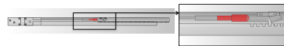
Figure 5 shows a Solidworks model of the jaws in the closed position. This position allows the jaws to be flush and fit through the trocar. The enlargement shows the plunger in the retracted position, to allow the top-jaw piece to form a 180° angle.
