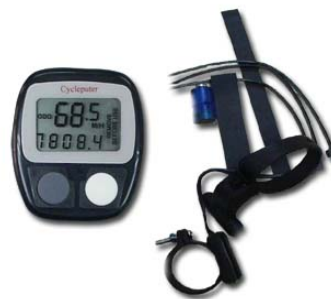
Figure 8: Bike speedometer with the equipment to count revolutions of a wheel. From http://image.made-in-china.com/2f0j00FeOEKtJhrRpj/Bicycle-Cycle-Computer.jpg
