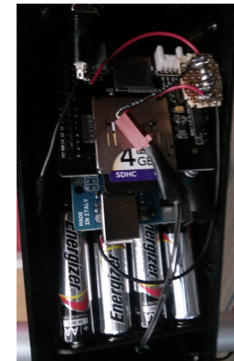
Figure 8. Microcontroller with SD card and battery modifications in mountable box.
