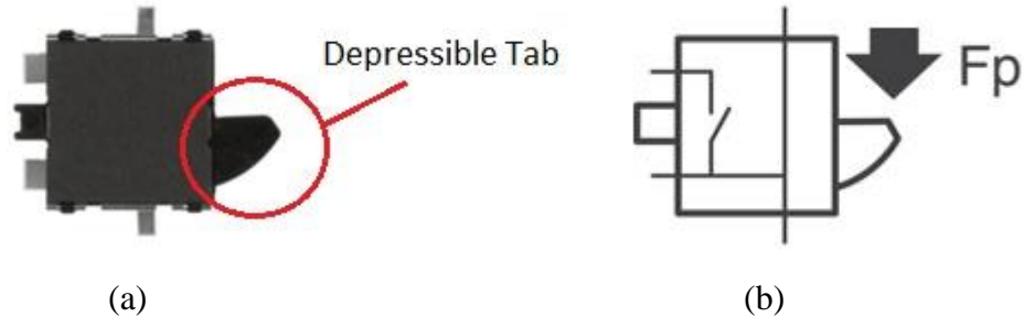
Figure 2: (a) The tab that is depressed when a cigarette is inserted (b) and the direction of the force applied and the completion of the circuit..
