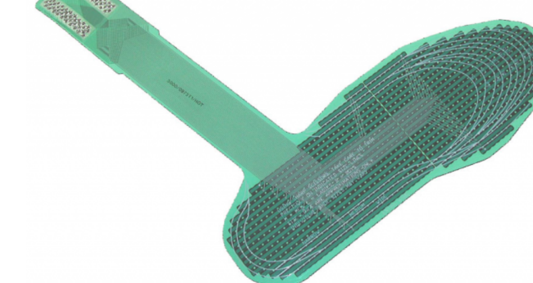
Figure 7: Tekscan pressure mapping system [3]
