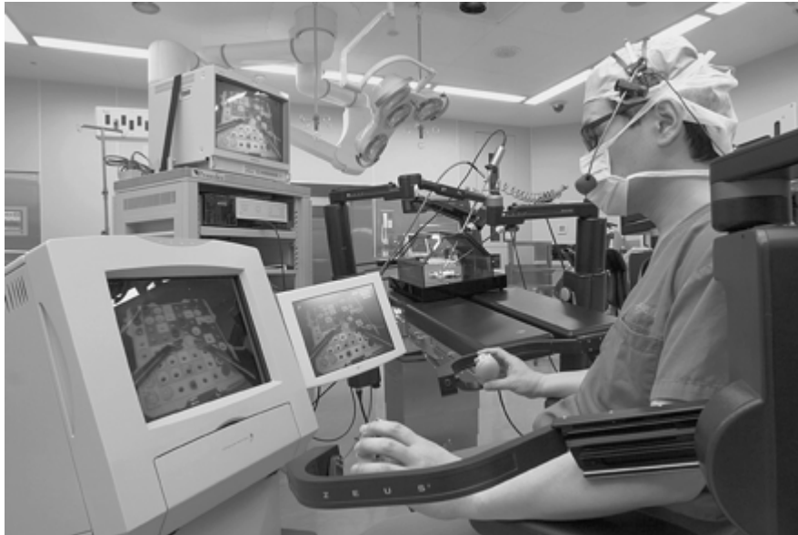
Figure 1: Setup of the ZUES Robotic Surgical System in a clinical setting ( http://www.ufrgs.br/imunovet/molecular_immunology/surgery_robotical.html ).
