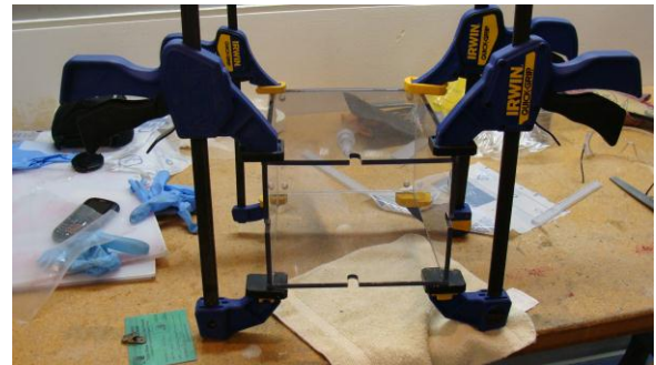
Figure 11: Cementing the outer box of the bioreactor.
