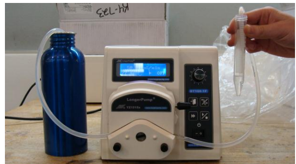
Figure 12: Pump testing set up.
