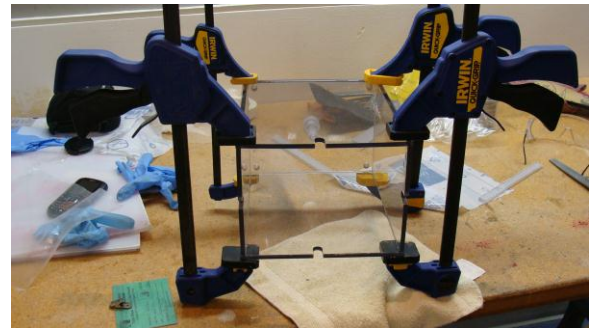
Figure 11: Cementing the outer box of the bioreactor.
