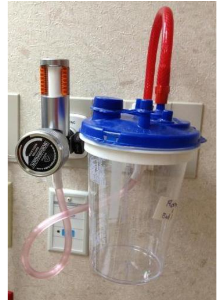
Figure 6: Photo vacuum pump used for collapse pressure testing.
