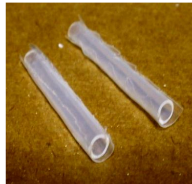
Figure 10: Photo of sample with 1 mm perforations with 2 mm spacing (left) and sample with 5 mm perforations with 2 mm spacing (right), demonstrating the bulging rough edge of the larger perforations and full expansion after sheath removal.
