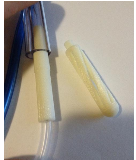
Figure 2: Picture of the 3-D printed tip and connector design.
