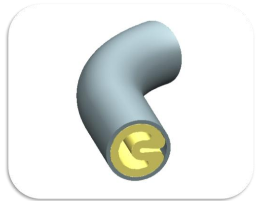
Figure 1: CAD model of the cross section of the first design alternative, showing a folding inner tube with a cleave
