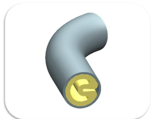
Figure 3: CAD model of the cross section of the first design alternative, showing a folding inner tube with a sleeve.
