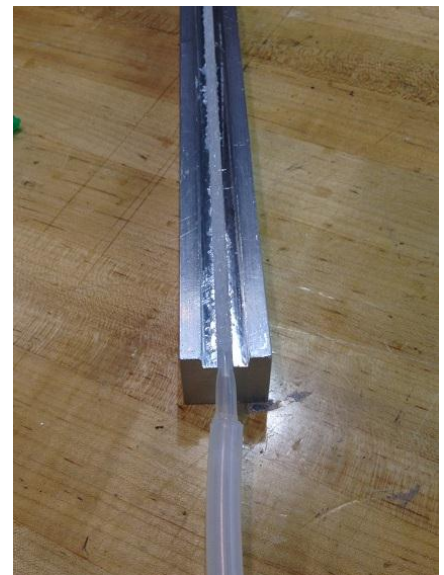
Figure 16: Picture of the constructed aluminum die.
