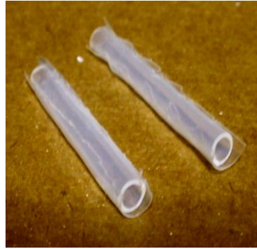
Figure 11: Photo of sample with 1 mm perforations with 2 mm spacing (left) and sample with 5 mm perforations with 2 mm spacing (right), demonstrating the bulging rough edge of the larger perforations and full expansion after sheath removal.
