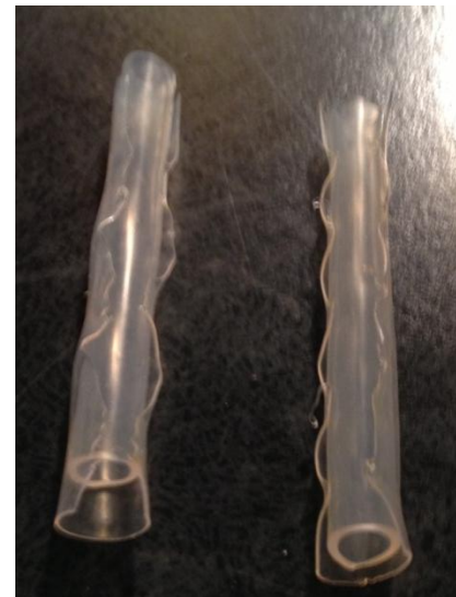
Figure 13: Pictures of sample heat shrink tubing tears with sharp edges. The perforations were closer together on in the tube on the right.
