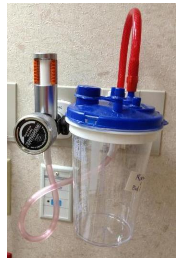
Figure 7: Photo vacuum pump used for collapse pressure testing.
