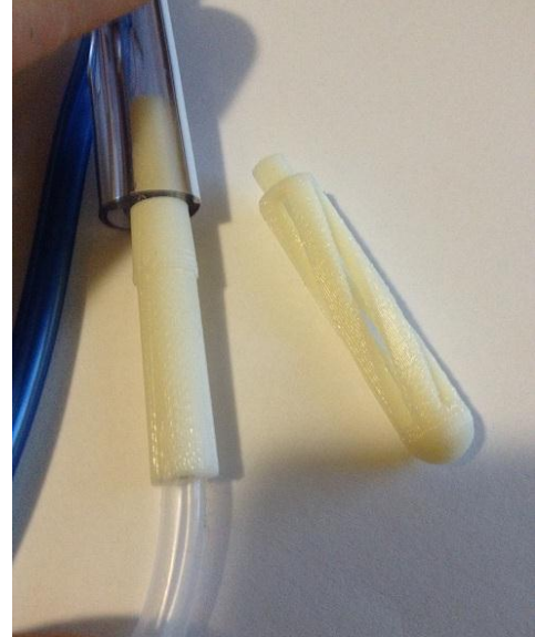
Figure 14: Picture of the 3-D printed tip and connector design.
