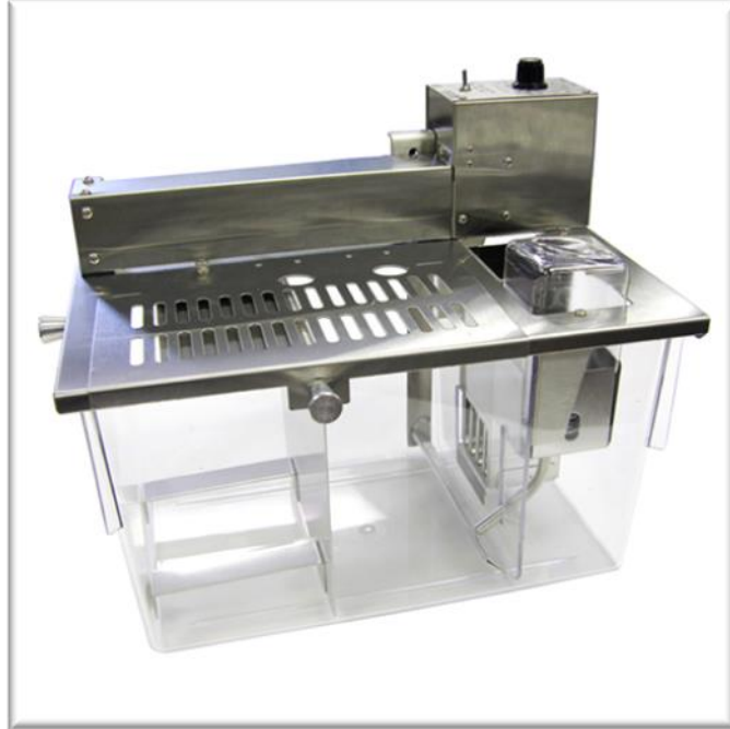
Figure 3 - Sleep deprivation chamber existing product: A device which features a sliding bar which is swept across the bottom of the cage forcing the mice to walk over it. (16)
