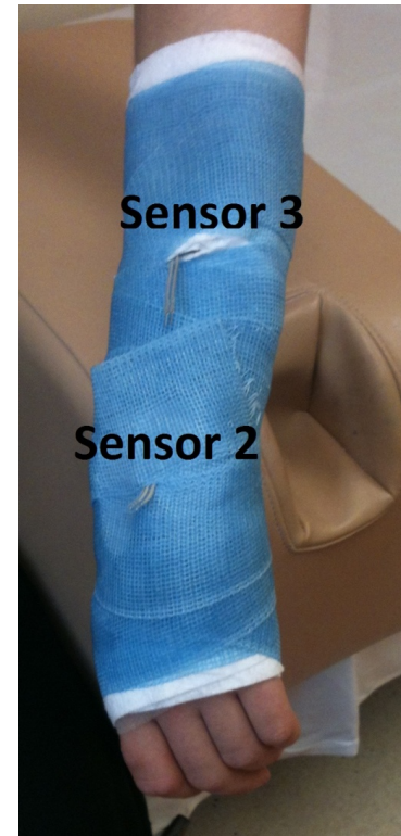
Figure 8: Dr. Halanski casted over sensors with leads exposed.
