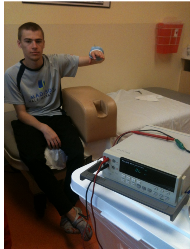
Figure 13: The multimeter is used to measure the resistance of the sensors.
