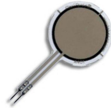
Figure 5 : This is the FlexiForce Sensor used.
