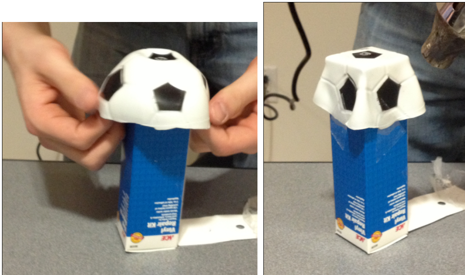
Figure 9: Before using the heat gun (left) and application of heat with the heat gun as the plastic forms to the shape of the box.
