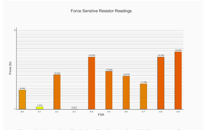
Figure 3: Processing displaying live bar graphs with force output for each sensor
