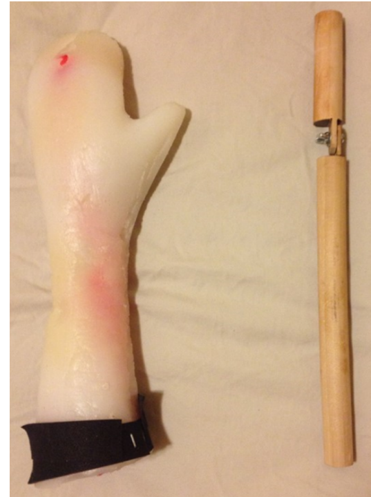
Platsil mold with 10 sensors (with bumpers) attached clustered around wrist
