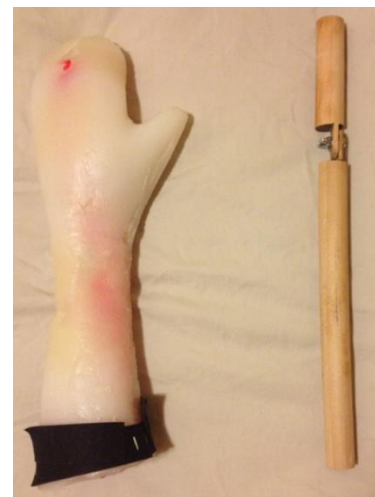
Figure 2: Platsil arm model and wooden dowel fracture system
