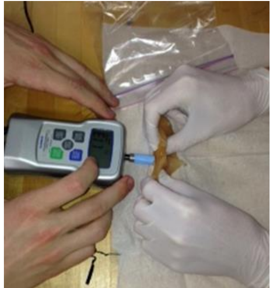
Figure 10: Chicken breast insertion force testing setup. The electronic force gauge was held steady as the 2cm thick chicken breast was pushed toward the gauge, with the needle completely penetrating the chicken breast.
