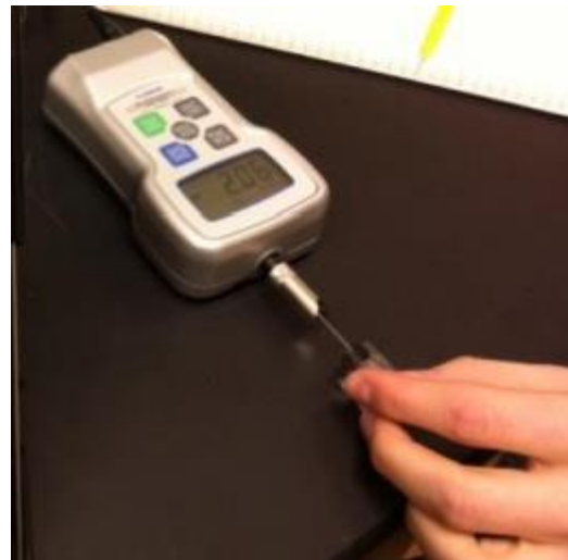
Figure 9: Testing setup for the single and double needle removal tests. The electronic force gauge was held steady while the clip was pushed slowly toward the force sensor.
