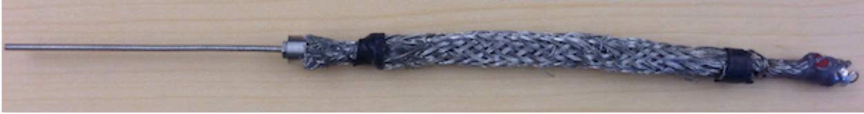
Figure 12: Completed prototype of design. The center threaded K-wire is attached to the bottom cap with JB Weld through the free-sliding top cap. The braid is attached with JB Weld to each cap. Another layer of braid was used to repair a braid rupture in the middle of the device due to damage sustained prior to fabrication. This repair braid was attached using heat shrink tubing. The threaded nut is above the top cap ready to compress the braid when driven by the drive shaft assembly.
