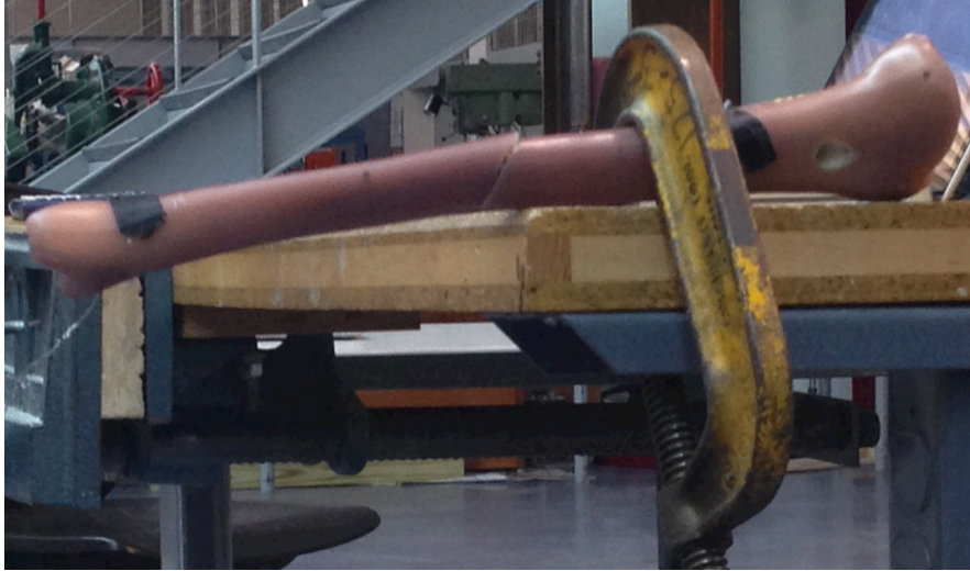
Figure 14: Cantilever bend testing setup.
