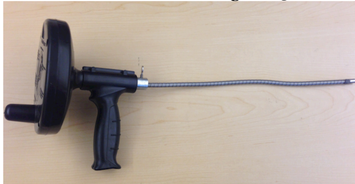
Figure 13: Drive shaft assembly for applying torque to nut above top cap on device from outside intramedullary canal. Consists of a manual auger (left), a segment of flexible hollow drive shaft (center), and the small external hexagonal broach serving as a socket adaptor used to engage the nut (right).
