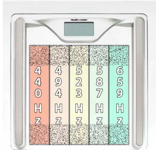
Figure 5. Conceptual diagram of second proposed design. Left/right zones are constant, but the plate vibrates in the front and the back when weight distribution shifts too far in those directions.
