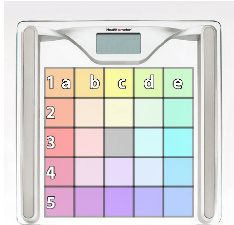
Figure 7. Conceptual diagram of fourth proposed design. Each zone is assigned two tones depending on left-right (x) and front-back (y) positions. Both tones play simultaneously to indicate two-dimensional weight distribution.
