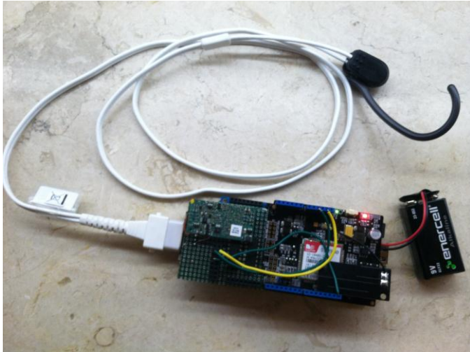
Fig. 1. Fully operational pulseMobile device. SeedStudio GSM Shield and Smith's Medical BCI board/sensor integrated with an Arduino Mega ADK powered by 9V battery.
