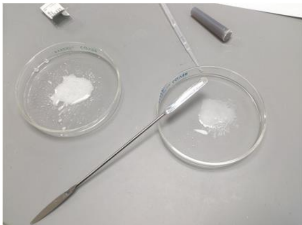
Figure 14: PEG in pill Absorbance Test. Both Hydrocodone and oxycodone were crushed, and then PEG was added drop-wise until pill was suspended.
