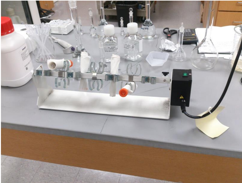
Figure B1: Tilting mechanism used for tilt method of testing The LabQuake machine constantly spun the samples around its axis, and solvent
