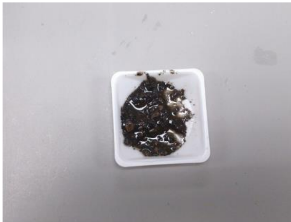
Figure 15: PEG in Sodium Bentonite Absorbance Test. Sodium bentonite was weighed, then PEG was added drop-wise until bentonite was suspended.
