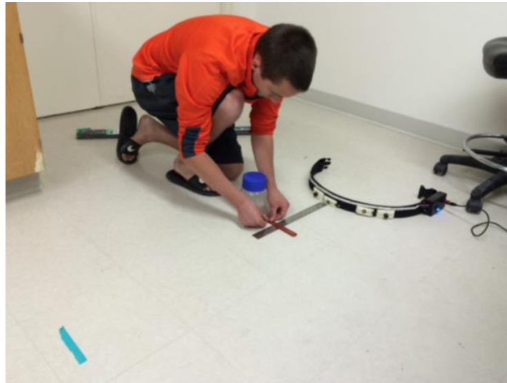
Figure 7: A demonstration of the testing procedure to measure the angle of the lateral viewing area of each sensor.
