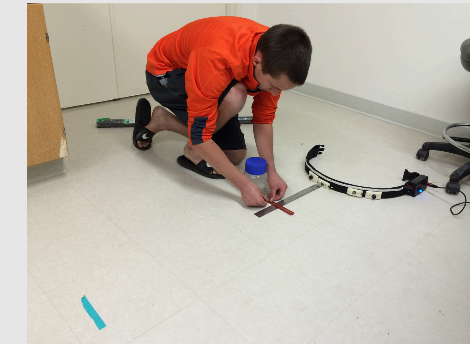
Figure 7: Field of view testing with one sensor pair.
