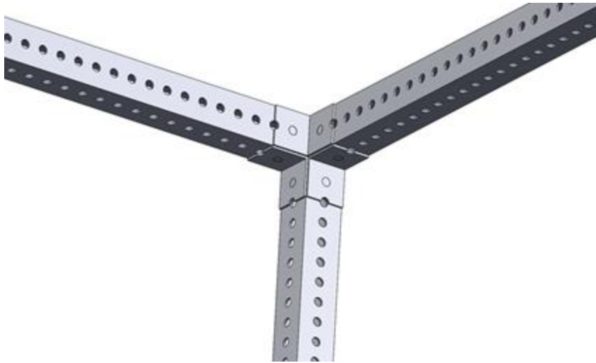
Figure 3: An image constructed in SolidWorks of the 90 degree metal fittings that join the struts of the U-Cube.
