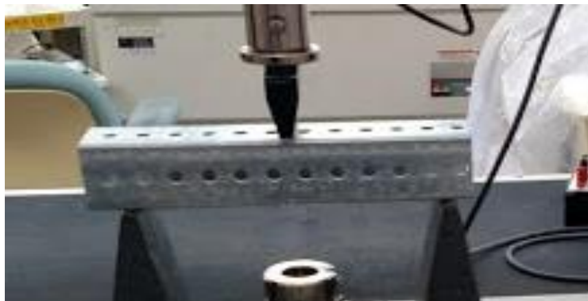
Figure 14: A sample being tested in three point bending on a Sintech 10,000 lb. MTS machine.
