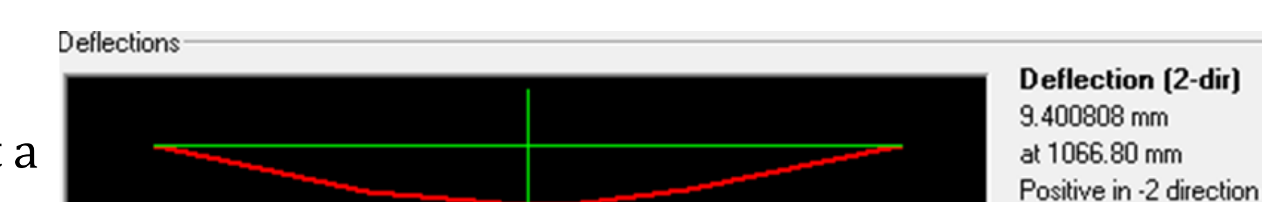
Figure 10a: SAP figure detailing deflection of a 2.13 m beam under 1780N beam centered load on an overhead beam
