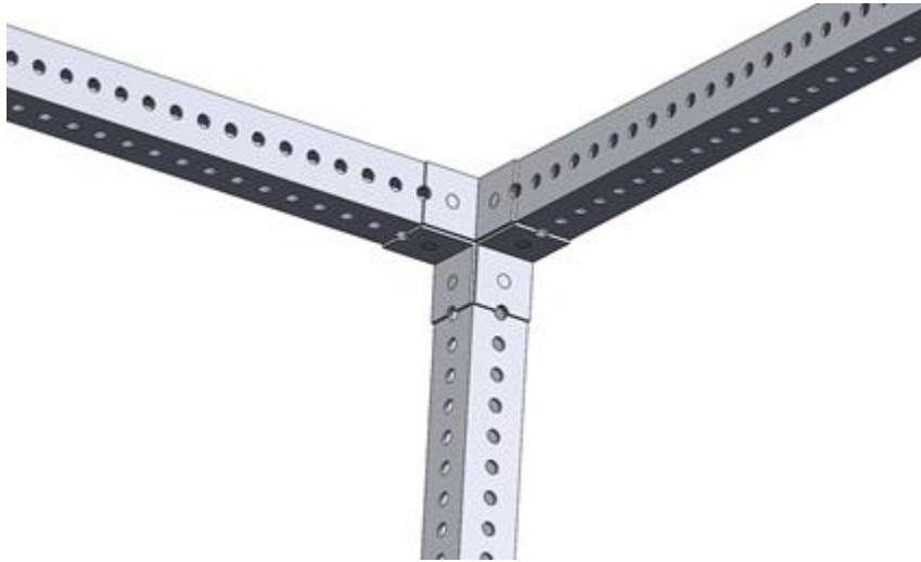
Figure 3: An image of the 90 degree metal fittings that join the struts of the U-Cube.
