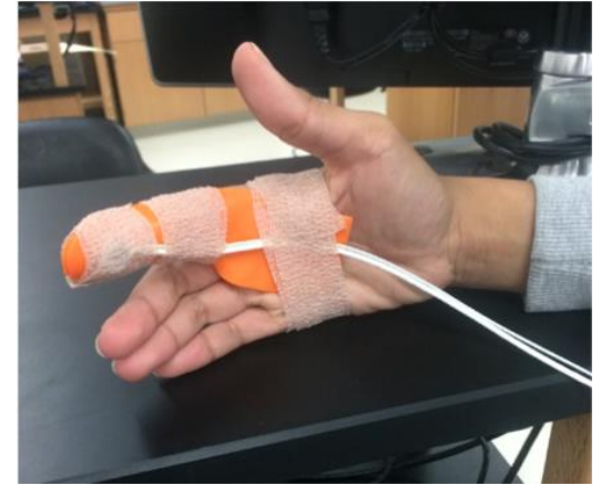
Figure 1. Splint device created in Fall 2015 to reduce noise on the blood pressure waveform.
